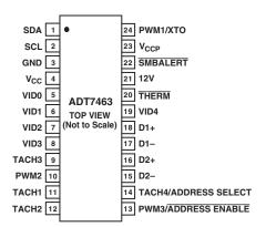
Figure 6. Pinout Option 5
