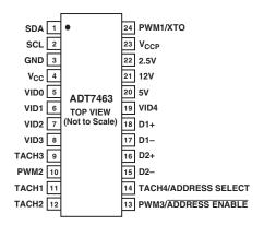
Figure 4. Pinout Option 3
