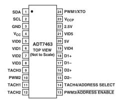
Figure 5. Pinout Option 4
