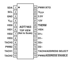
Figure 7. Pinout Option 6
